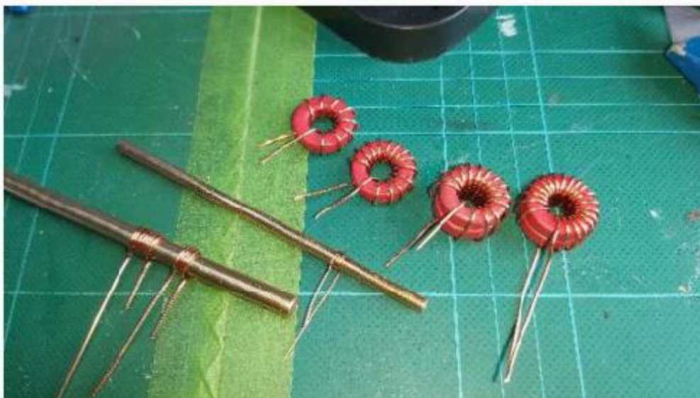
Inductor winding with brass mandril
