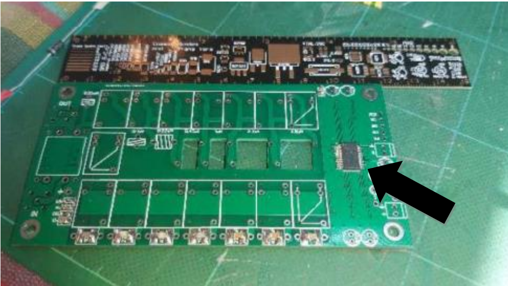
7x7 Auto ATU bare board (sigh of relief after most nervewracking component attached) 6 inch ruler used for reference.
